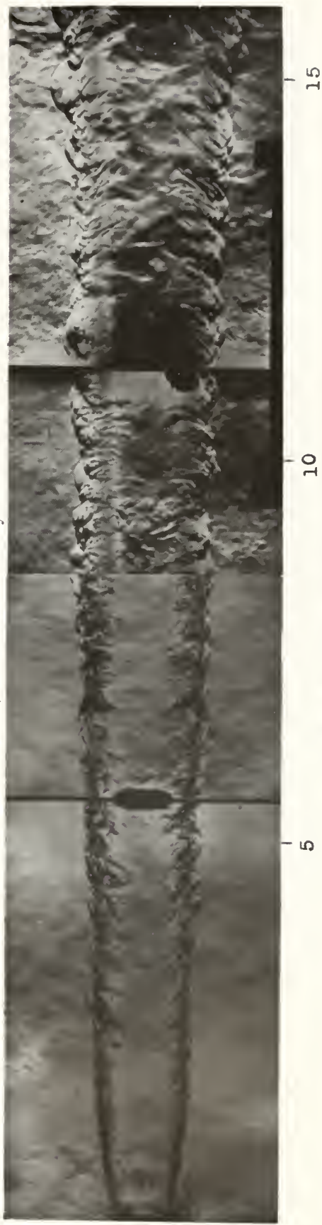
Figure 10. Composite Photograph of Flame Spreading from 1 inch Diameter Flameholder; \phi = 1.0 , 300 ft/sec Mixture Velocity
